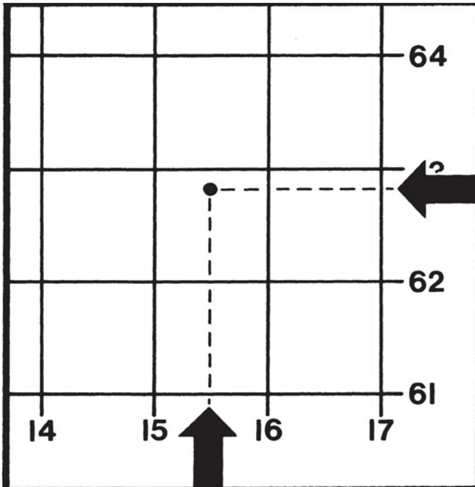
*The point marked with a dot can be described as 15.5 x 62.8 using the coordinates from the sides of this grid. This system requires that squares are mentally divided into tenths in each direction. The 'map reference' is normally expressed as six digits: 155628. Any letter area codes on the map should be included.*
